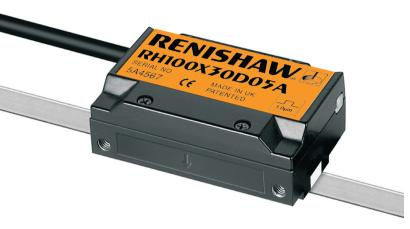
The RH100 readhead works with 40 µm reflective tape scale, has patented filtering optics, set-up LED, and offers high speed performance.
